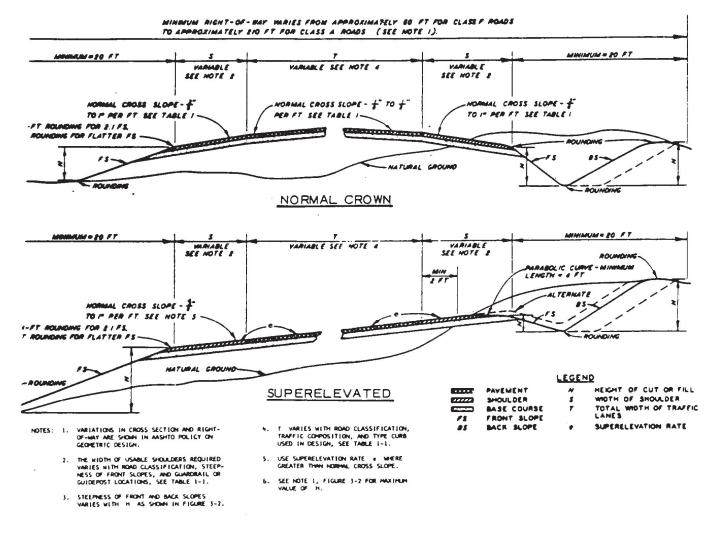
Figure 3-6. Typical road-type cross sections.
